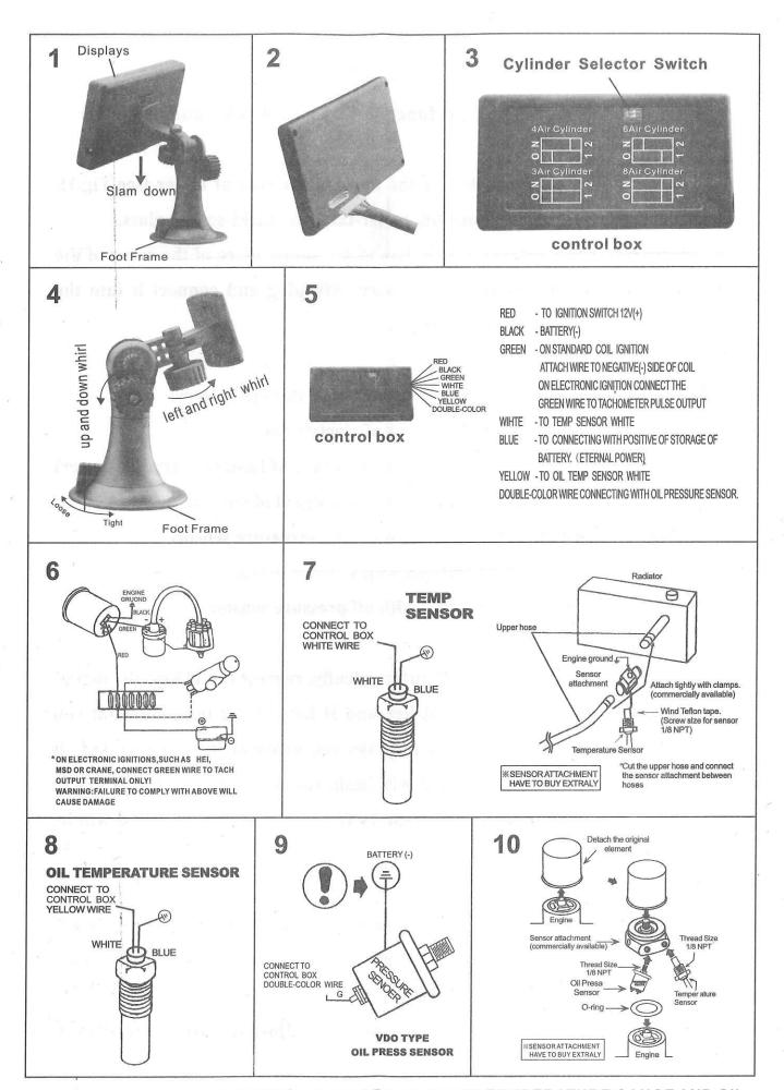
ATTENTION: SENSORS OF WATER TEMPERATURE GAUGE AND OIL TEMPERATURE GAUGE ARE UNIVERSAL.
